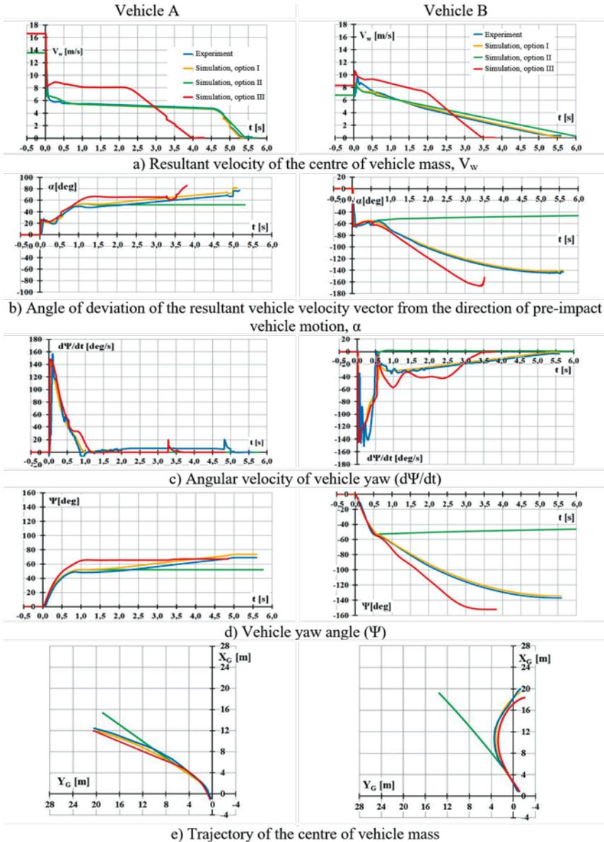
Fig. 6. Comparison between experimental and simulation test results for test Z3
