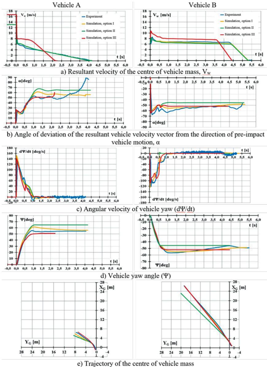
Fig. 7. Comparison between experimental and simulation test results for test Z4
