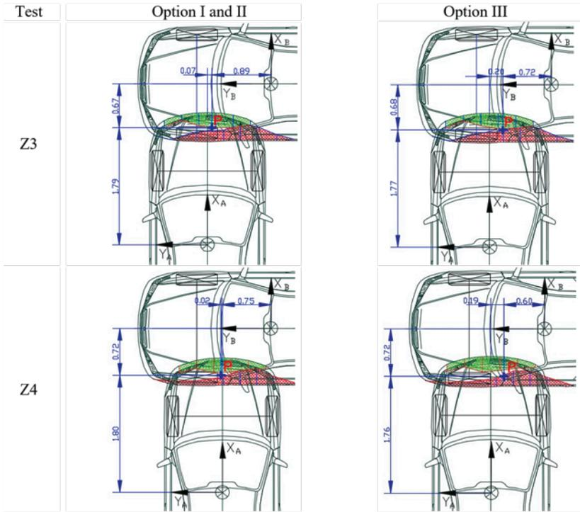
Fig. 5. Determining the coordinates of the point of application of the force impulse (point P) for the three options of the input data applied in the vehicle collision simulation tests
