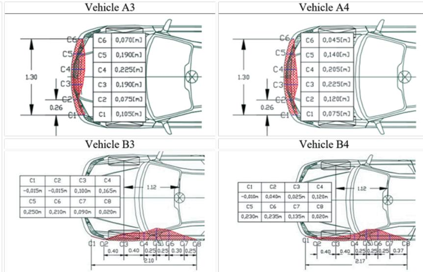
Fig. 4. Permanent deformations of the vehicles involved in tests Z3 and Z4
