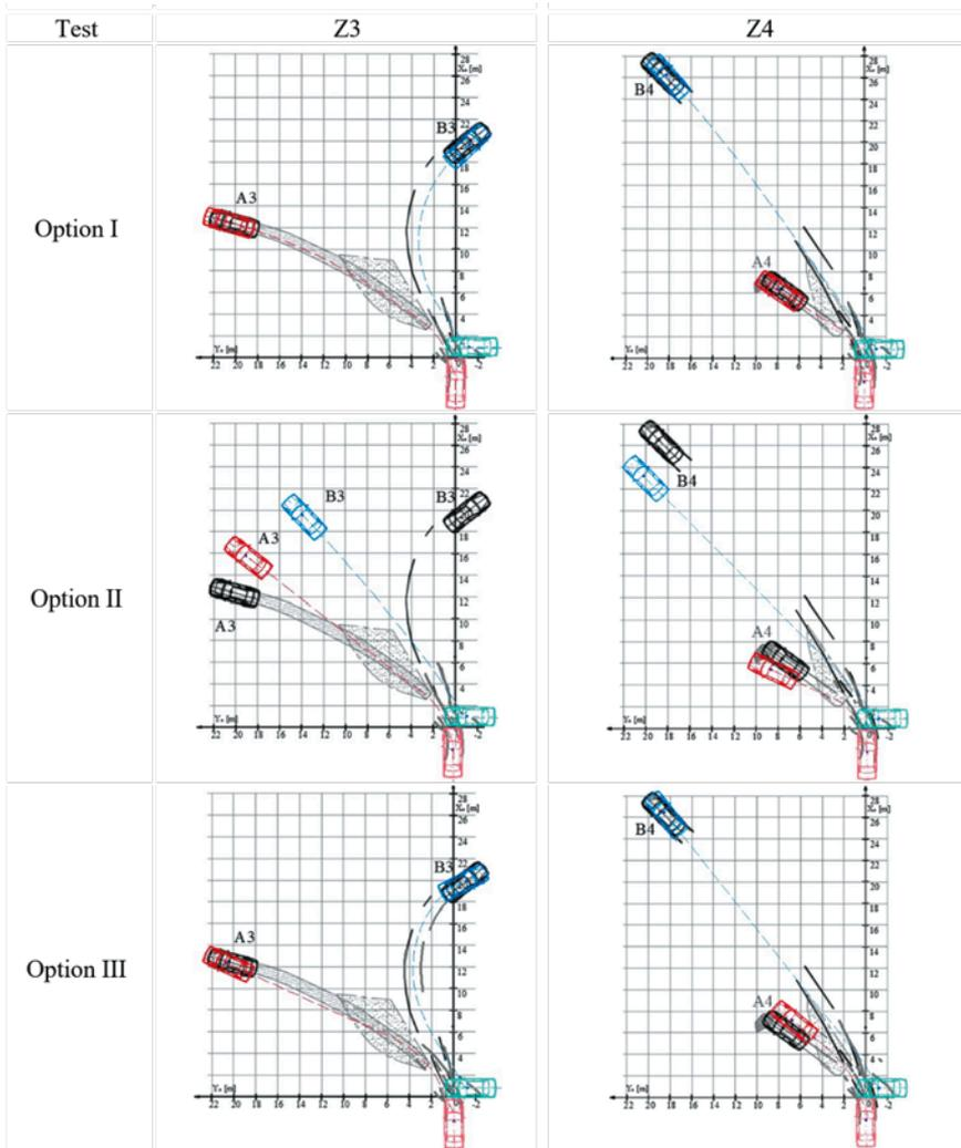
Fig. 8. Post-impact rest positions of vehicles A and B and wheel scuffmarks made on the road during the experiment (drawn in black) and obtained from the simulation (red for vehicle A and blue for vehicle B) for the three options of the input data
