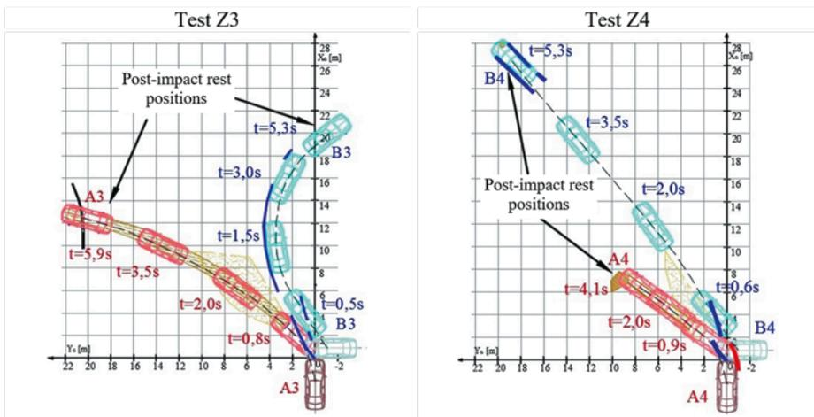
Fig. 1. Marks left on the road in result of the collision in tests Z3 and Z4
