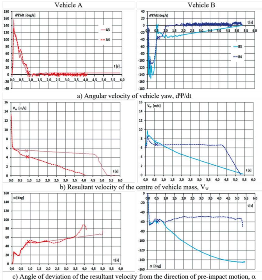
Fig. 3. Time histories of the values of the parameters of motion of vehicles A and B in tests Z3 and Z4
