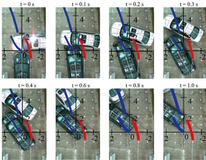
Fig. 2. Mechanism of the wheel scuffmarks being made during test Z4
